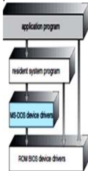
Figure 2.8 MS-DOS layer structure.
